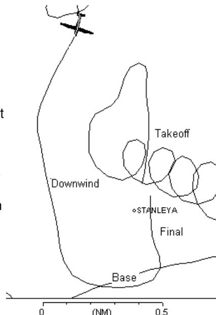
how quickly the glider loses altitude during landing. On base the sink is 900 ft/min. This and more can be derived from the GPS track. It is very useful for routine analysis of flights - especially good for students to practice improving their circuits, etc.
