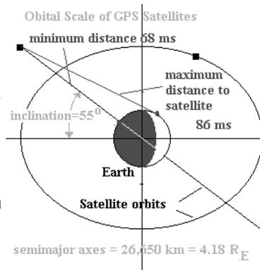
fifty-five degrees with respect to the equatorial plane. This constellation guarantees the user of five to eight SVs visible from any point on the earth. The orbit altitude (22,000 km) is such that the satellites repeat the same track and configuration over any point approximately each 24 hours (4 mins earlier each day). Orbital period is 12 hours.
