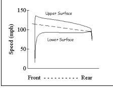
along the wing. The mean airspeed of the air around the wind is 100 mph.
